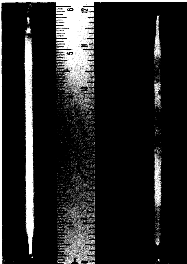
Fig. 10.1. A sample of pure \text{UF}_6 sealed in glass is on the left-hand side and impure \text{UF}_6 containing chromium or nickel fluoride impurities is on the right-hand side.
